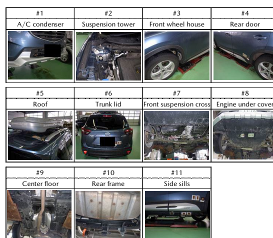
Fig. 4 Environment Measuring Point
