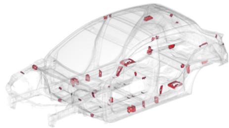
Fig. 9 Applied Location of Damping Stiffener (red painted)
