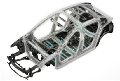
Fig. 1 Body-in-white of Mazda3 with Damping Control Structures Using Structural Adhesive (light blue line)
