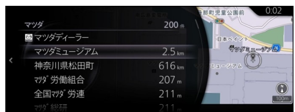
Fig. 18 Search Results and Map Pane: Right Tilt will Change Control Pane to Adjust Destination
