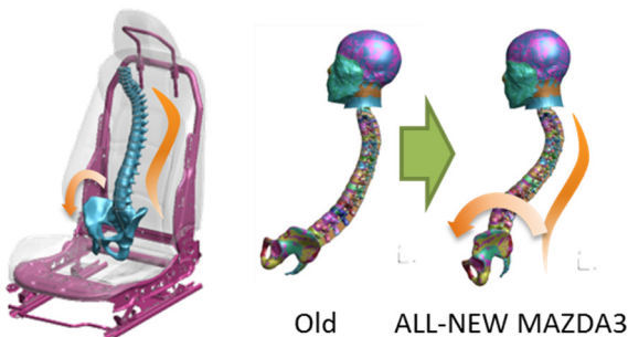
Fig. 7 New Seat Structure & S-Shaped Alignment of Spine
