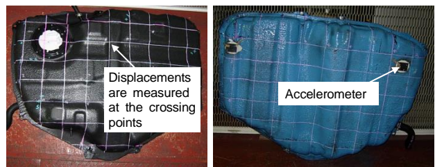
Fig. 14 Grid Lines for 3-D Measurement
