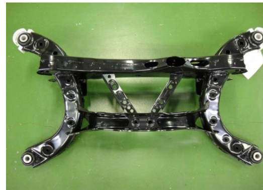
Fig. 12 Appearance of Sus-crossmember by New Anti-corrosion Process
