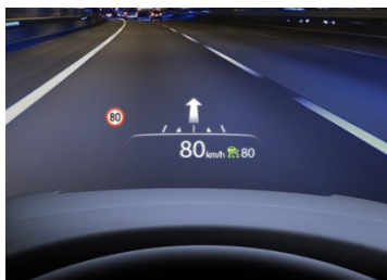
Fig. 15 Active Driving Display Front Window Shield Type
