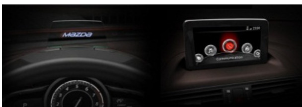
Fig.16 Active Driving Display &amp; Center Display
