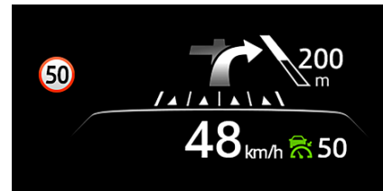
Fig. 20 Traffic Signal Recognition System
