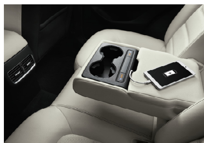
Fig. 12 Air Condition Vents & Two USB Charging Ports
