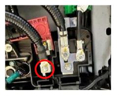
12) Wear insulating gloves and remove front connector and attached wiring harness clip.
