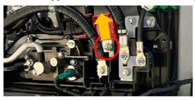
(14) Remove cooler pipes and attached wiring harness clip.
