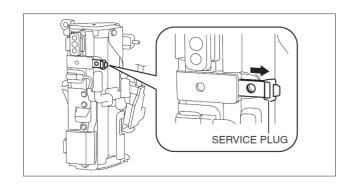
7. Using the removed installation bolt, fix the service plug at the position to which it was pulled out.
