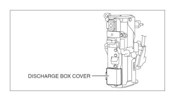
9. Connect the connector in the discharge box to the plug as shown below.
