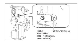
6. Pull the service plug in the direction of the arrow shown in the figure.
