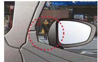
Pillar and side mirror shape that minimize blind spots
