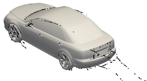
Fig. 2 Vortex Core Line Method
