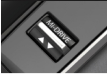
Fig. 4 Switch of Mi-Drive
