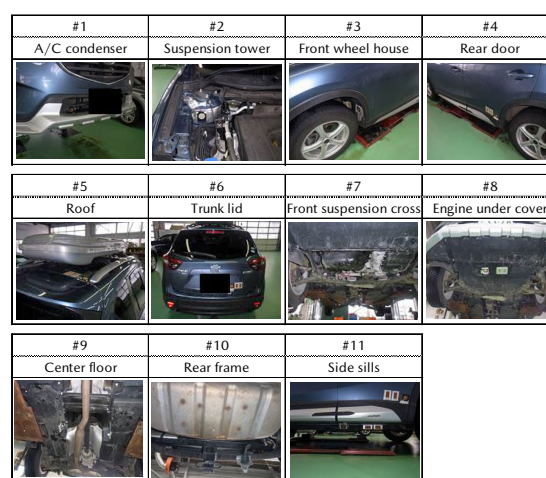
Fig. 4 Environment Measuring Point
