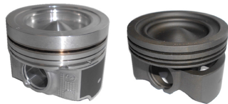
Fig. 11 Previous-Aluminum Piston (Left) New-Steel Piston (Right)
