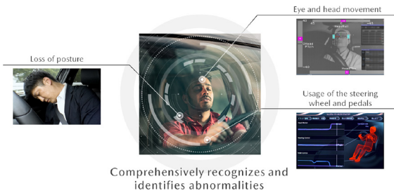
Fig. 10 How the System Monitors the Driver's Condition
