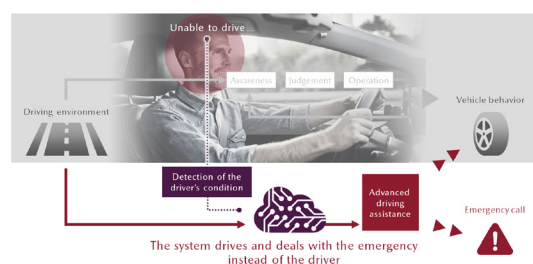
Fig. 9 The System Drives and Deals with the Emergency Instead of the Driver
