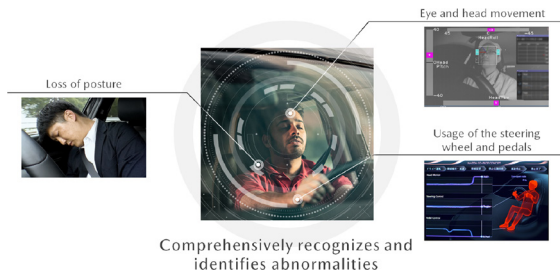
Fig. 10 How the System Monitors the Driver's Condition
