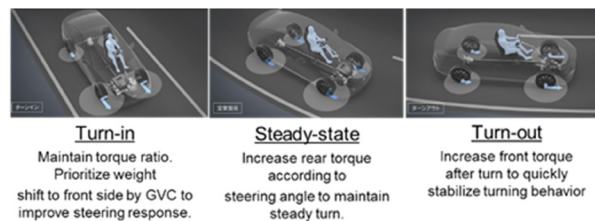
Fig. 3 AWD Torque Ratio at Turn
