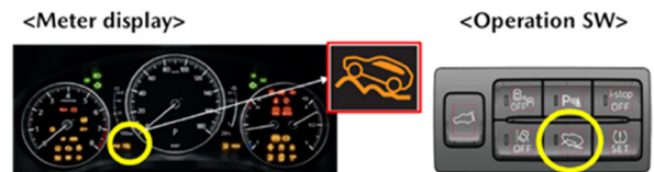
Fig. 8 Operation SW and Meter Display
