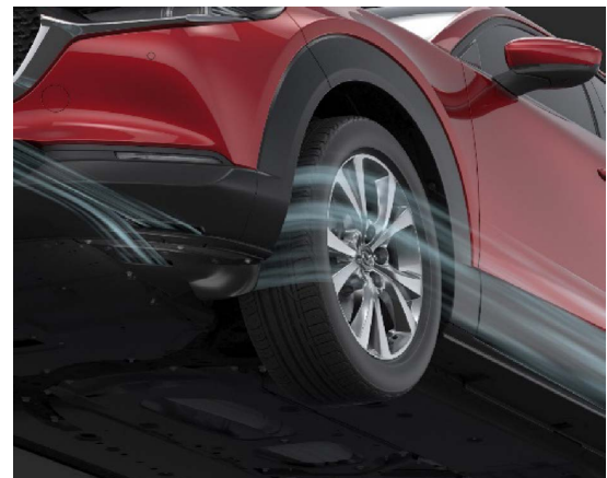
Fig. 25 Aerodynamic Optimization around Tire of CX-30
