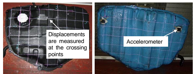
Fig. 14 Grid Lines for 3-D Measurement
