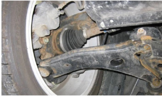
Fig. 1 Chassis Condition after Vehicle Corrosion Test
