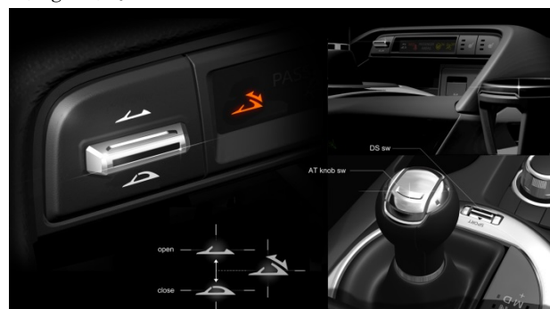
Fig. 14 Roof Operation Switch
