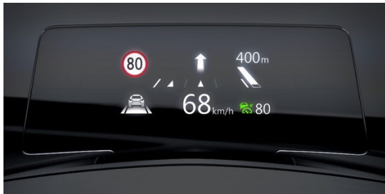
Fig. 8 Traffic Sign Recognition System
