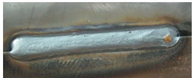
Fig. 15 Welding Bead by High-Ar Welding Process
