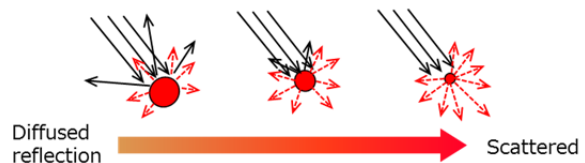
Fig. 12 Diffused Reflection Depend on Pigment Size
