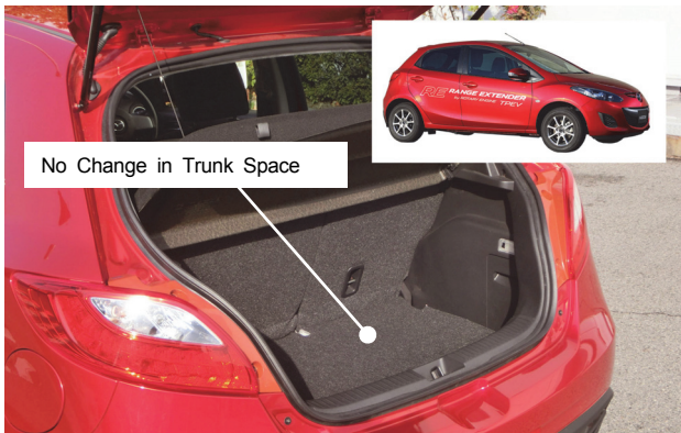
Fig. 3 Demio EV, Range Extender Unit Installed
