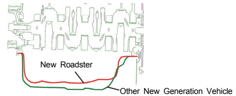
Fig. 17 Lower Oilpan Height of SKYACTIV-G
