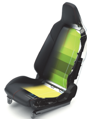
Fig. 6 Seat with New Structure
