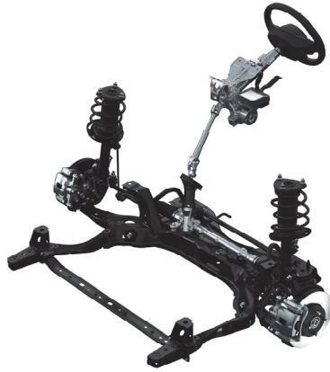
Fig. 1 Front Suspension and Steering
