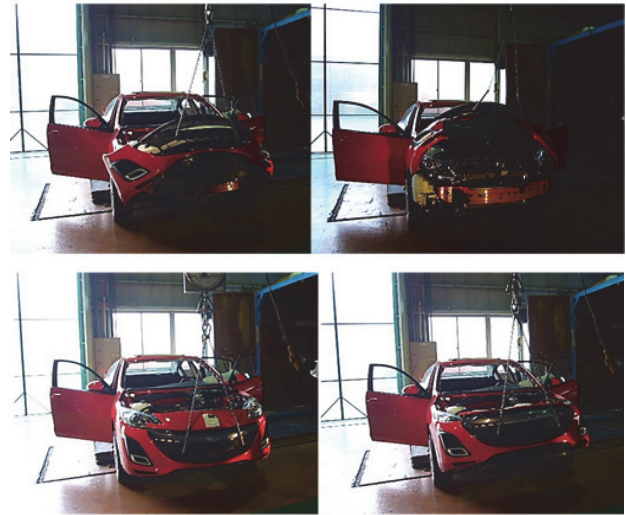
Fig. 9 Dismantlement Test of Bumper Designed for Recycling
