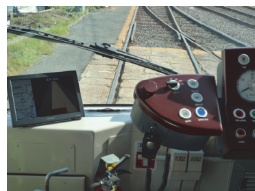
Fig. 11 Support Monitor for Tramcar
