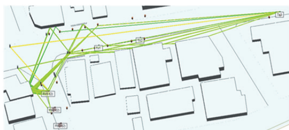
Fig. 4 Simulated Propagation Paths (TX3-RX1)
