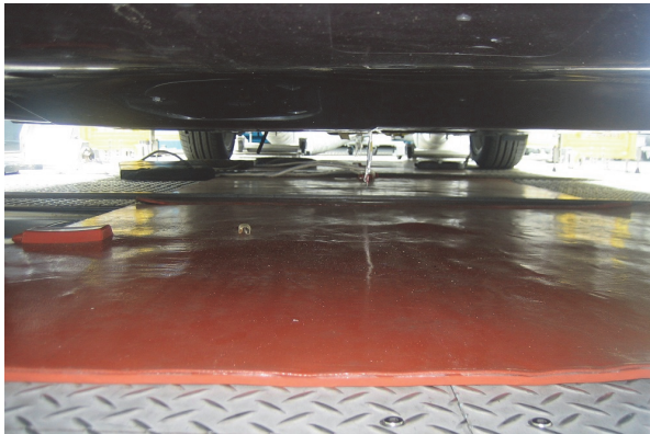
Fig. 4 Heat Mat for Appropriate Floor Temperature
