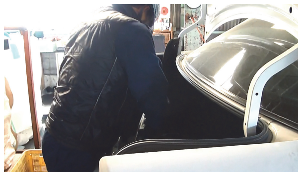
Fig. 4 Dismantlement Test 1 of Rear Bumper of Mazda Familia (Remove Trunk Mat)
