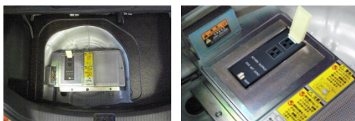
Fig.12 100V Electric Supply System
