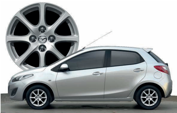
Fig.6 14inch Light Weight Aluminum Wheel
