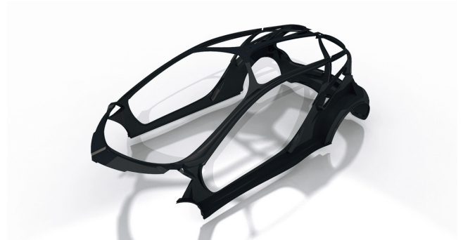
Fig.7 Upper Body Structure of KIYORA
