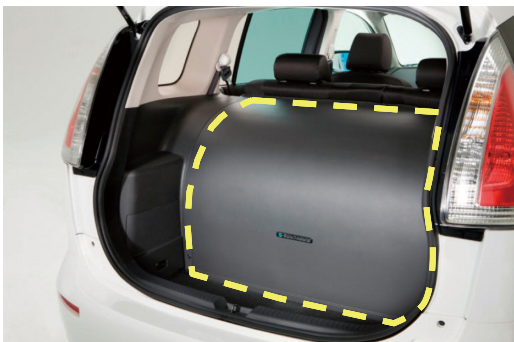
Fig.12 H 2 Tank Cover on Premacy Hydrogen RE Hybrid
