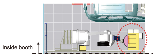
Fig.7 Space Saving Cartridge System
