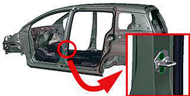
Fig.7 Double Latch for Sliding Door
