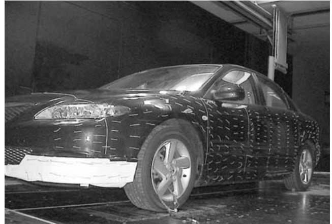
Fig.2 Air Flow Analysis around Upper Body in Wind Tunnel
