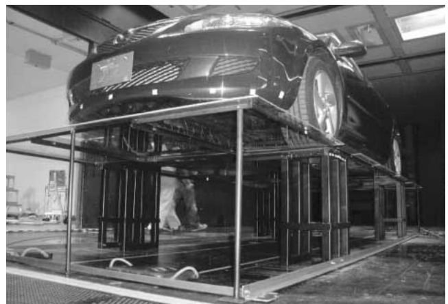
Fig.3 Equipment for Under Floor Flow Analysis
