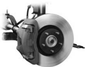
Fig.5 17" Front Ventilated Brake
