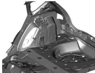
Fig.9 Reinforcement at Suspension Tower-Rear
