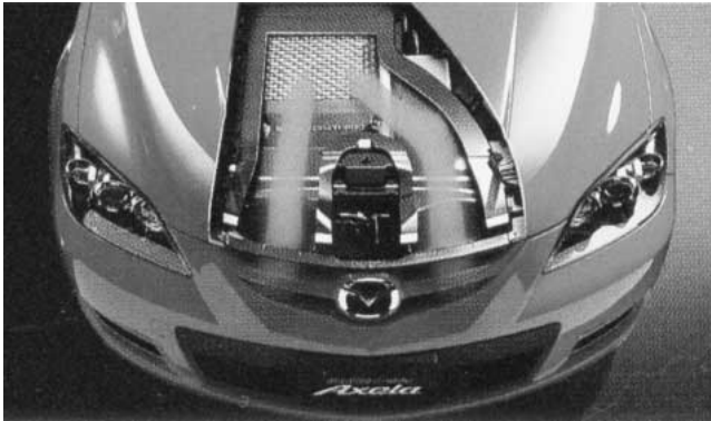
Fig.12 Inter Cooler Duct Structure
