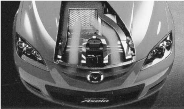
Fig.12 Inter Cooler Duct Structure
