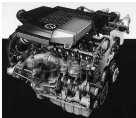
Fig.1 MZR 2.3L DISI Turbo Engine
