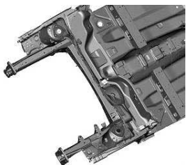
Fig.8 Reinforcement at Cowl-Front
