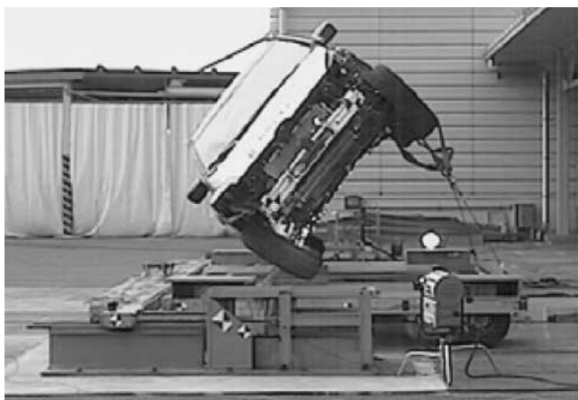
Fig.14 Trip Over Test
