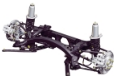
Fig.10 Multilink Rear Suspension
