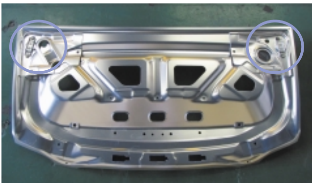
Fig.15 Appearance of Reinforcement Assembly
