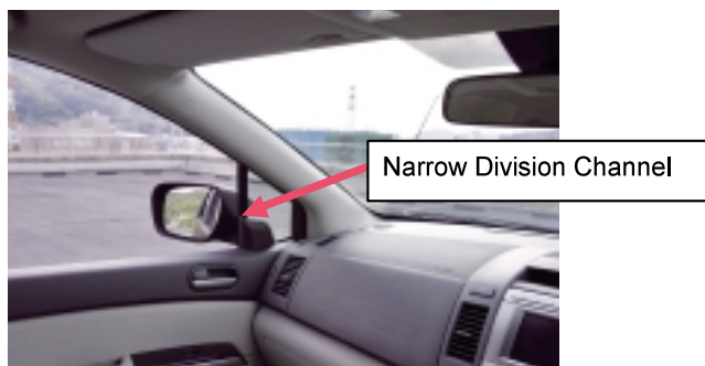
Fig.20 Triangle Window and Division Channel
