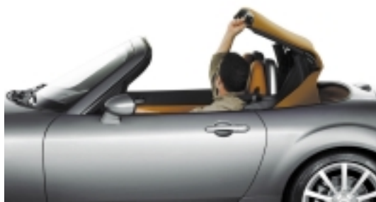
Fig.11 Z-fold Design Soft Top for Easy Opening and Closing
