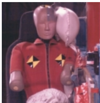
Photo of Sled Test at 18ms
