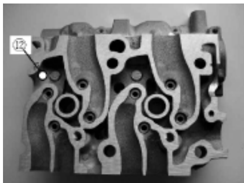
Water jacket upper deck side
