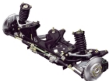
Fig.9 Double Wishbone Front Suspension
