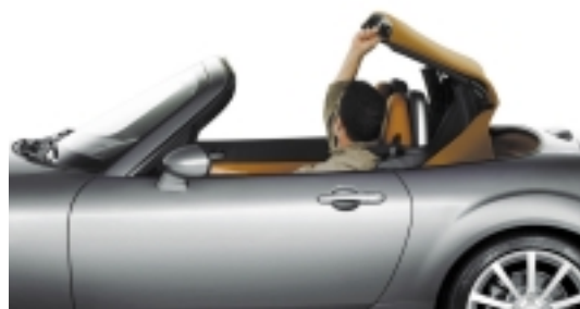
Fig.11 Z-fold Design Soft Top for Easy Opening and Closing
