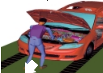
Fig.3 Double Slat Conveyor (Conventional)
