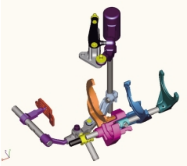
Fig.4 Internal Change Mechanism
