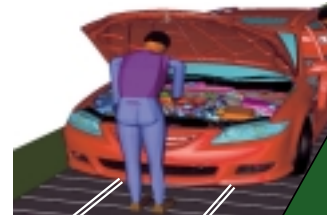
Fig.4 Triple Slat Conveyor (Reborn)
