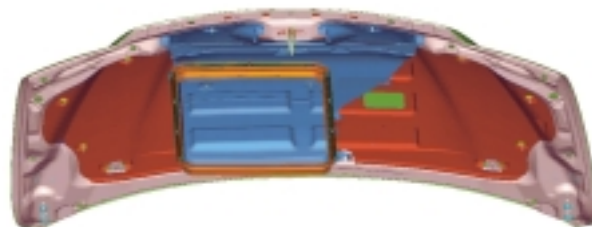
Fig.17 Air Duct behind a Hood
