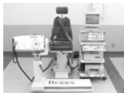
Fig.3 Measurement Devices of Ankle Joint Torque
