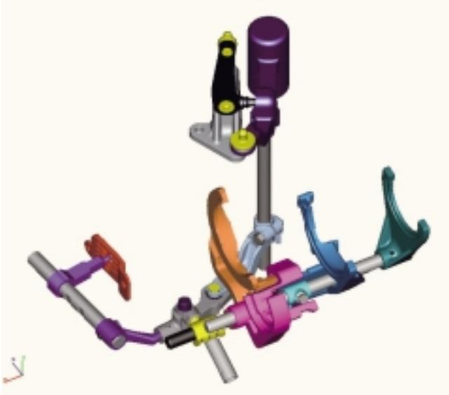
Fig.4 Internal Change Mechanism
