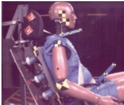
Fig.12 Sled Test with Steel Rigid Seat
