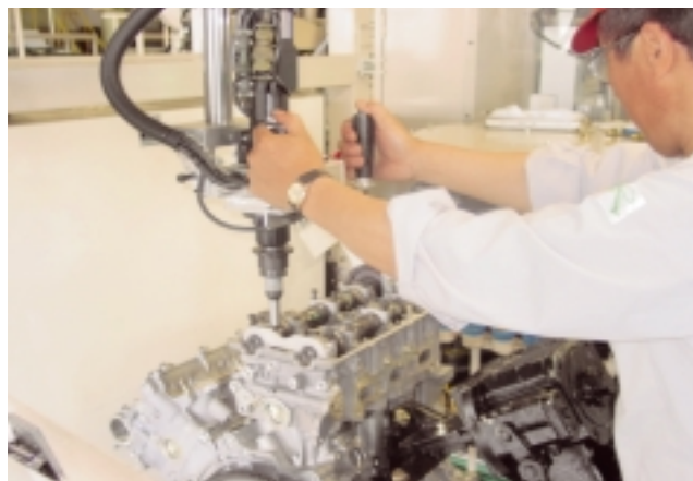
Fig.5 Nutrunner for High Torque Use
