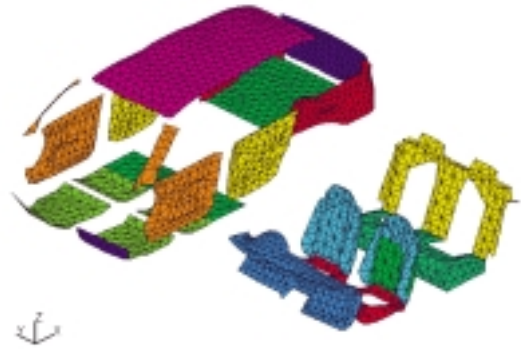
Fig.11 Acoustic Impedance Setting Parts
