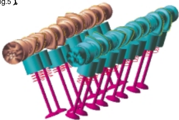
Fig.4 Valvetrain Dynamics Model
