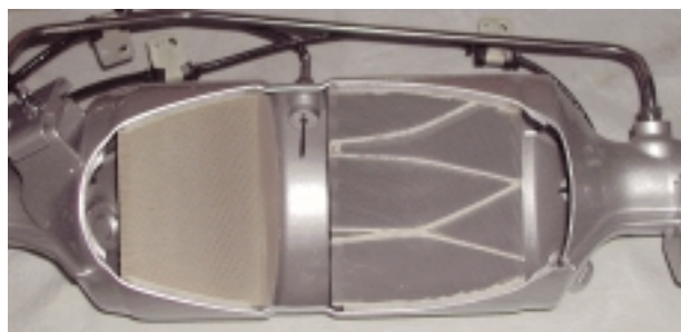
Fig.7 DPF Unit (cut model)
