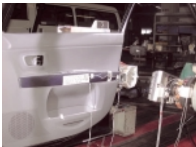
Fig.8 Door Impact Test
