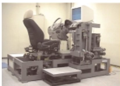
Fig.1 Driving Operation Task Creation Simulator
