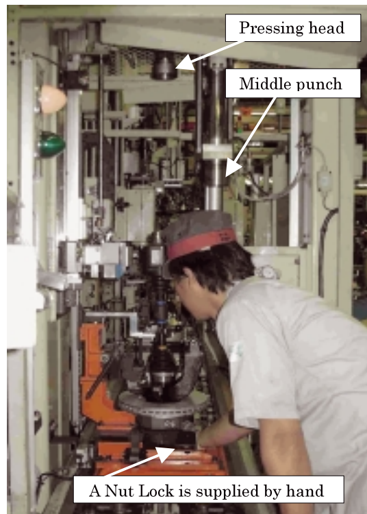
Fig.5 Drive Shaft Assy Press Fitting
