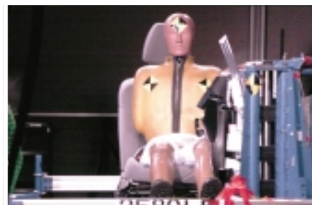
Fig.7 Side Impact Crash Simulator
