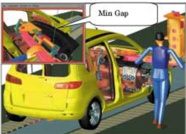
Fig.13 Evaluation of Visibility at IPM Install
