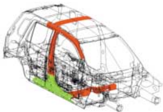
Fig.5 High Energy Absorption Body Structure for Side Impact
