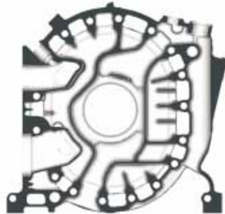
Fig.19 Section of Intermediate Housing
