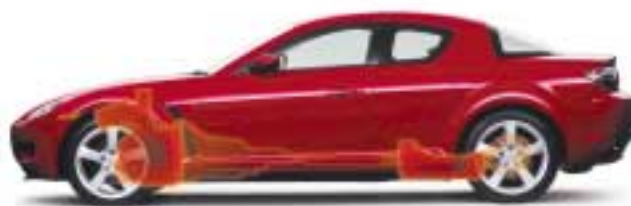
Fig.4 Advanced Front Mid-ship Layout
