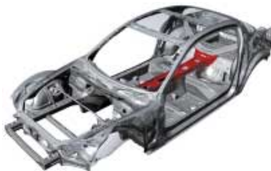
Fig.15 Body Structure Complete
