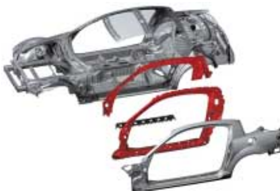
Fig.17 Cab-side Structure with T.W.B. Parts
