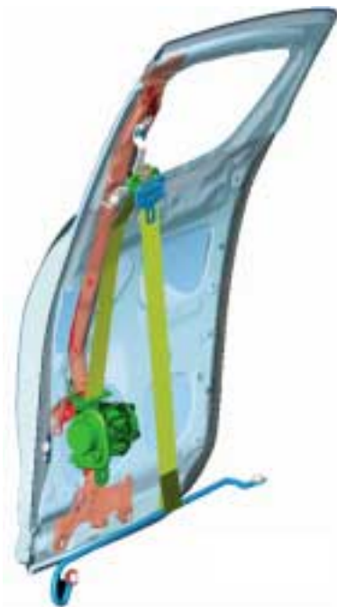
Fig.12 Front Seat Belt Installation
