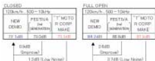
Fig.12 Wind Noise Level (Wind Tunnel Test)
