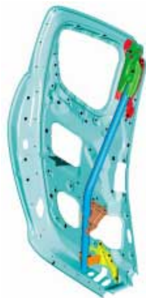
Fig.10 Built-in Pillar Structure
