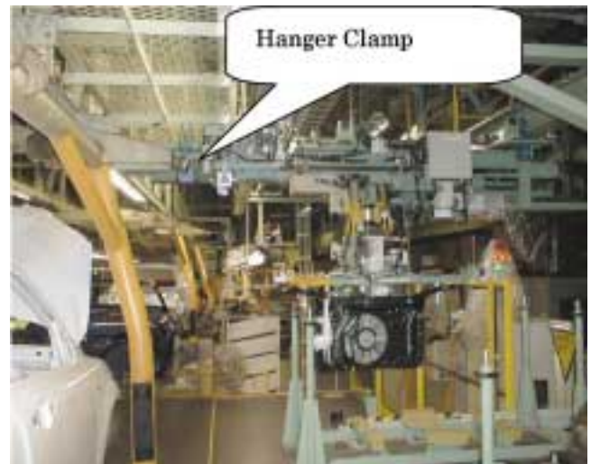
Fig.3 Hanger Clamp for FEM Install
