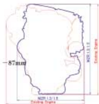
Fig.22 Overall Height and Width of Engine
