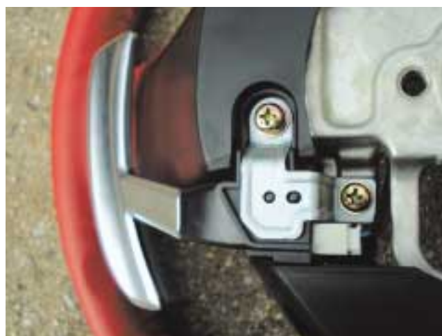
Fig.16 Structure of Metal Bracket
