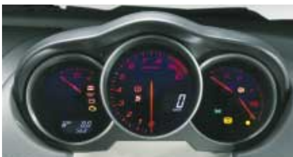
Fig.15 Night Illumination of Meter
