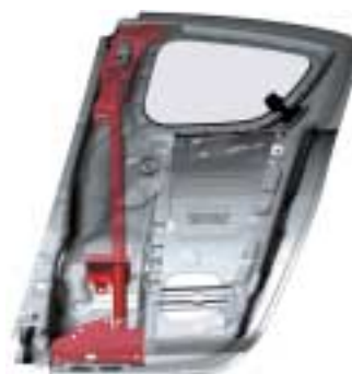
Fig.2 High-tensile-steel Pipe Reinforcement
