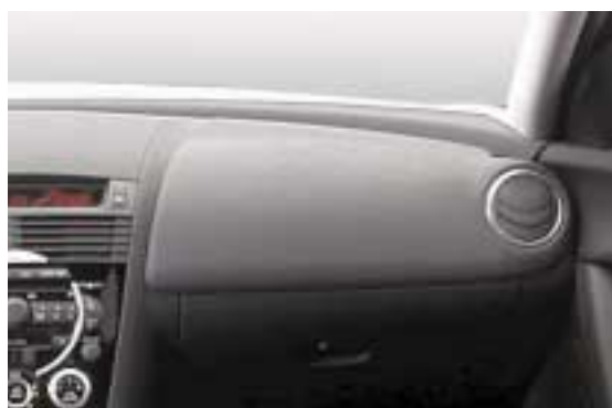
Fig.9 Seamless Airbag of RX-8
