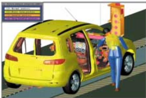
Fig.12 Evaluation of Work Posture at IPM Install
