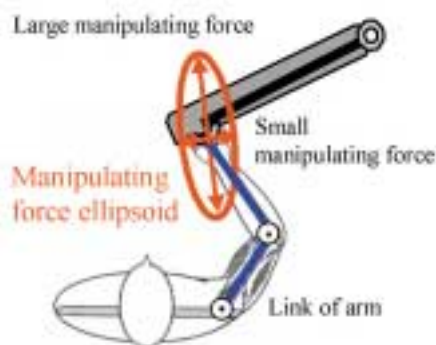
Fig.1 Manipulating Force Ellipsoid
