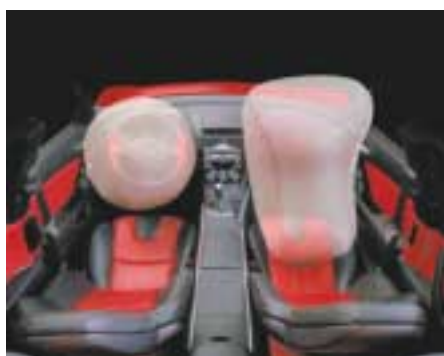
Fig.11 Dual Stage Frontal Airbags
