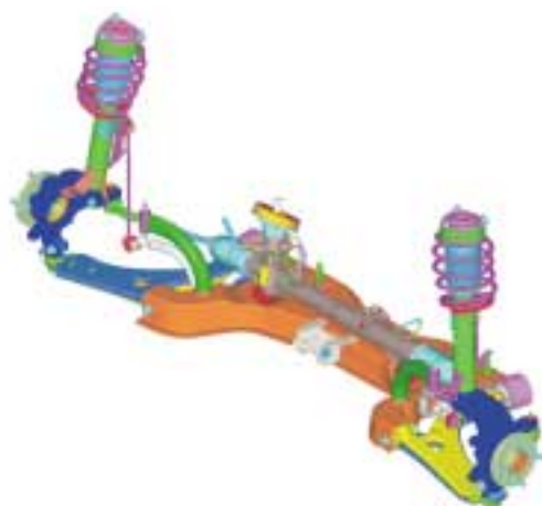
Fig.1 Front Suspension & Steering
