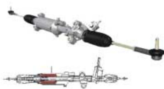
Fig.3 Rack-drive Type Electric Power Steering System
