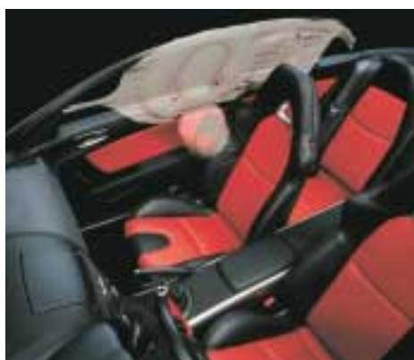
Fig.7 Side Airbag and Curtain Airbag
