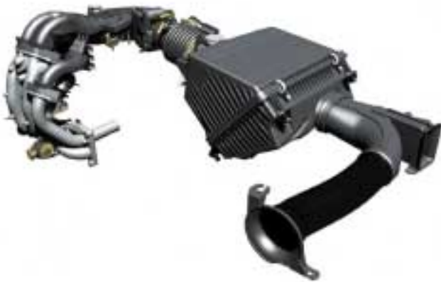
Fig.12 S-DAIS (Sequential Dynamic Air Intake System)
