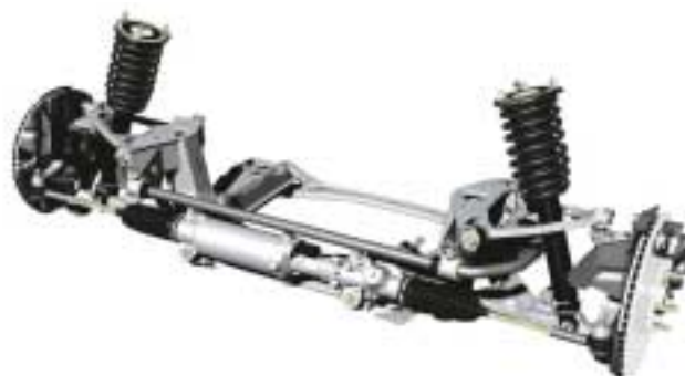
Fig.6 Front Suspension System
