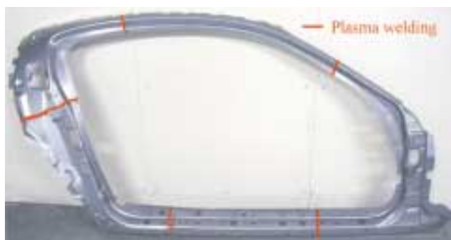
Fig.14 Forming Panel of RX-8 Side Flame Rain
