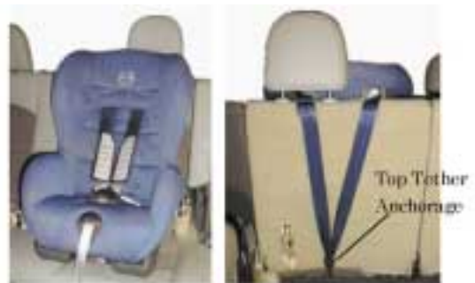
Fig.11 ISO-FIX Child Seat Top Tether Anchorage
