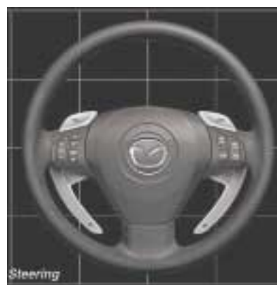
Fig.11 Design Proposal of Long Length UP Switch
