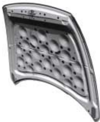
Fig.14 Pedestrian Head Protection Hood
