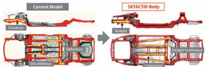
Fig.3 Straightening of Basic Framework and Continuous Framework Structure
