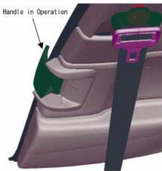
Fig.14 Rear Door Release Handle
