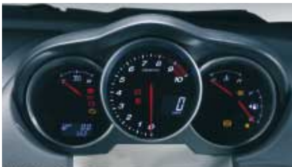
Fig.14 Day Illumination of Meter
