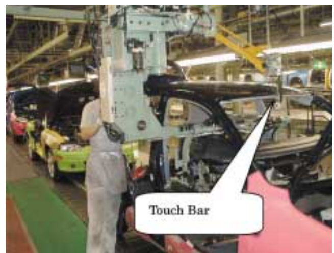
Fig.4 Conveyor Following at IPM Install
