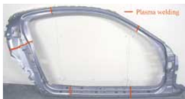
Fig.14 Forming Panel of RX-8 Side Flame Rain
