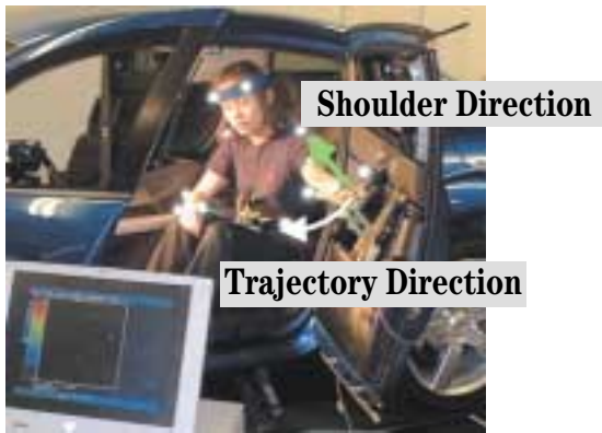
Fig.15 Door Operation Test
