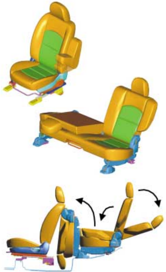
Fig.15 Seat & Rr.seat Double Folding
