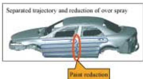
Fig.9 Reduction of Over Spray
