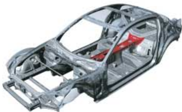
Fig.5 High Mount Back Born Frame
