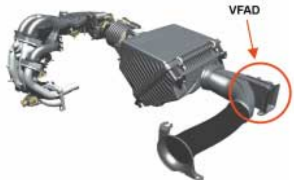
Fig.12 Variable Fresh Air Duct
