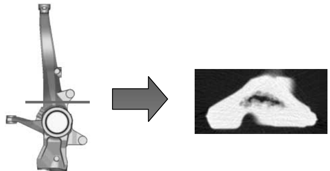
Fig.3 Shrinkage Form Section & CT Scanner Image
