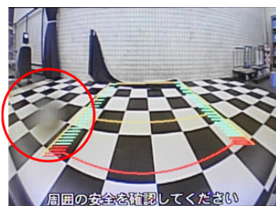
②Blur Caused by Water Droplets
