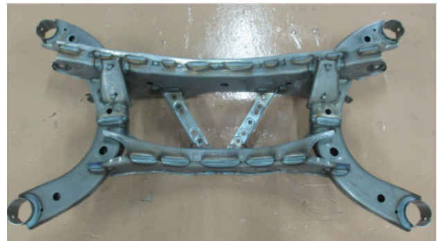
Fig. 14 Appearance of Sus-Crossmember by High-Ar Welding Process
