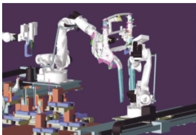
Fig.5 Spot Welding Without Using Jig
