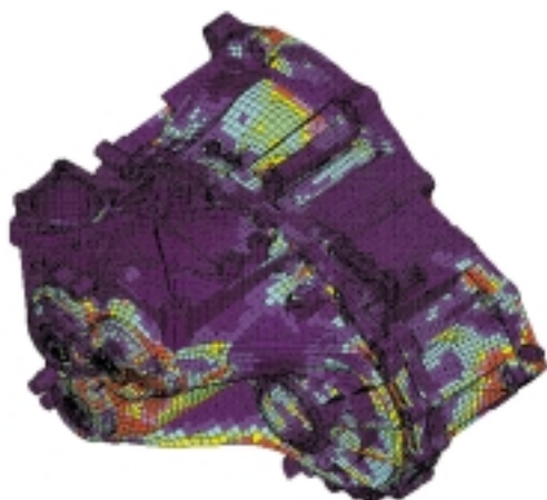
Fig.26 Case Vibration Analysis
