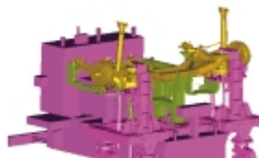
Fig.9 Rear Suspension Assembly to Accommodate Multi-Models
