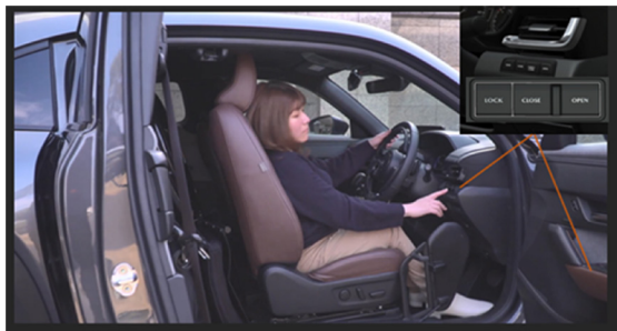
Fig. 11 Operation Switch Layout (2 places)
