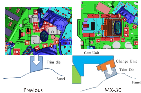
Fig. 4 Difference between Previous and MX-30 Structure
